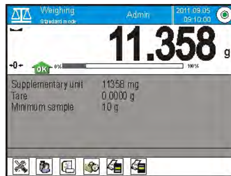
Weight value higher than the MSW value specified for a particular tare range.
